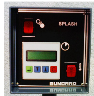
Control panel with new timer
