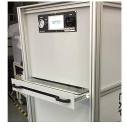
Press the vacuum button. The button will turn green and the vacuum pump will start running. Within a few seconds, the pump will have evacuated the air between the frame and the plate. The vacuum indicator will show approx. 0.8 bar.
