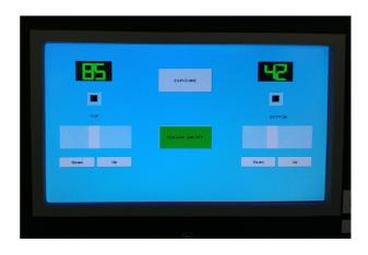
After everything is set and controlled, insert the drawer into the machine and press the **exposure** button. The lamps will light on and the timer(-s) will count down.
