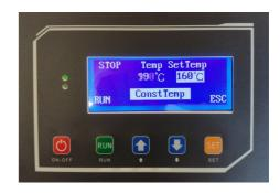
When the set temperature is reached, the indicator changes to green and the oven keeps the temperature.
