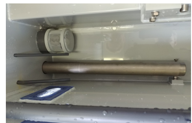
View on heater, pump filter, thermo-sensor and thermal fuse
